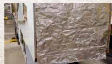
R-38 Radiant shield Thermo-foil wrap through ceilings, underbellies and under front caps.
