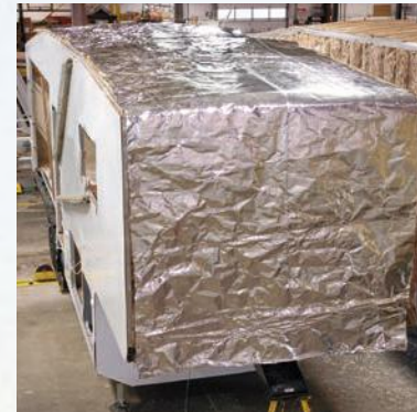
R-38 Radiant shield Therma-foil wrap through ceilings, underbellies and under front cap.
